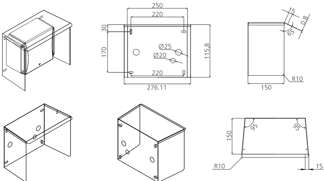
Note: the fire safety switch cannot be installed in the place with direct sunlight, and the sun visor is recommended.
